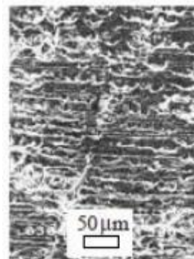
Figure 2.17. Chemical wear instance for cast iron because of the sulphuric acid [44].
