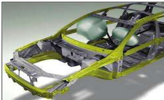
Figure 2.1. Example of DP steels as safety details in car bodies.
