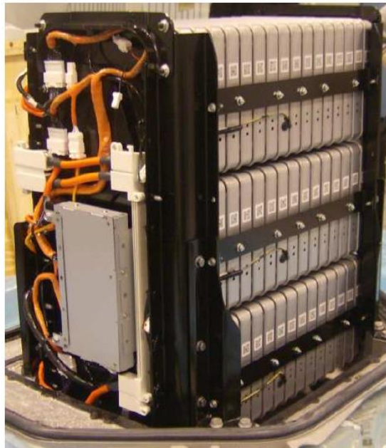
Figure 3.5. Li-Ion battery assembly (vertical) [19].
