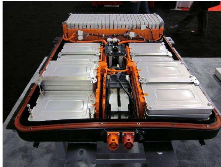
Figure 3.7. Li-Ion battery assembly (horizontal) [19].
