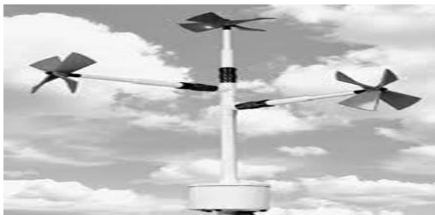
Figure 1.5. Propeller anemometers in fixed three-dimensional arrangement.
