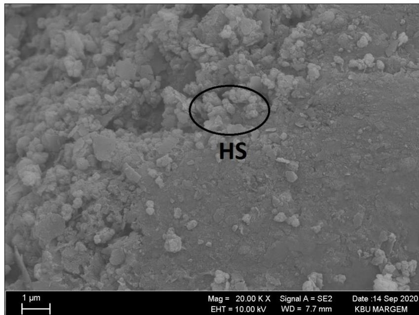
Figure 5.25. Microstructure of 10wt.% waste glass added samples. K; kaolinite, HS ; Hydrosodalite.
