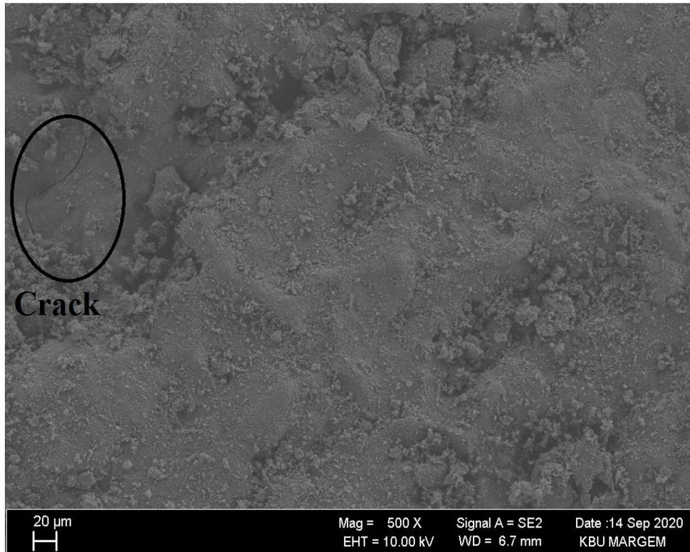
Figure 5.22. Microstructure of 40wt.% Metakaolin added samples.
