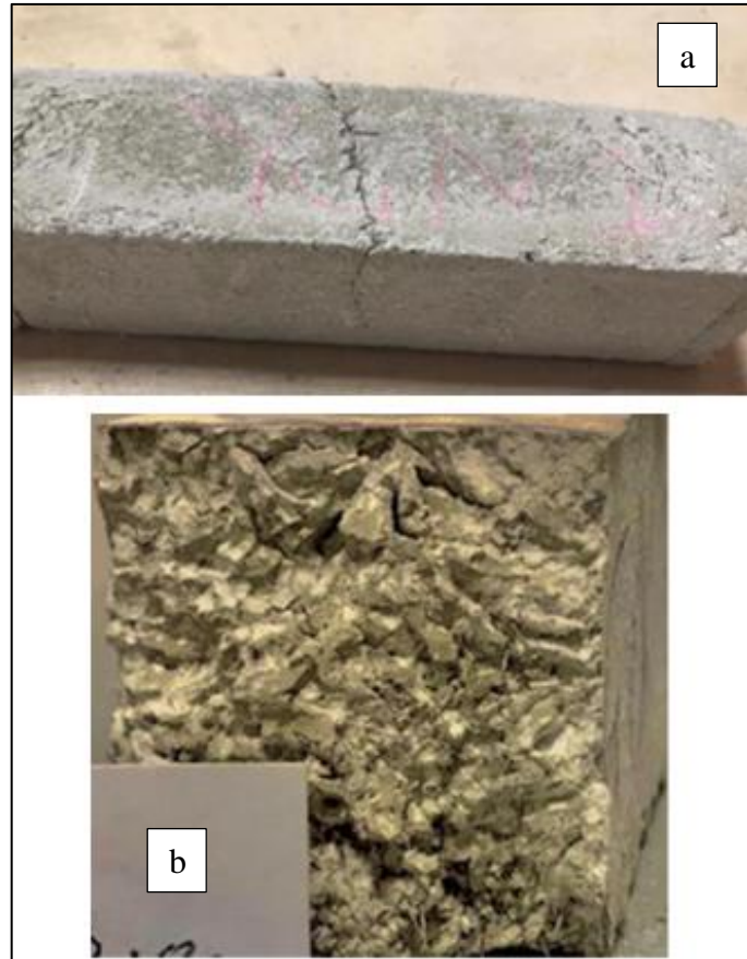
Figure 4.11. a) GSN2 batch after the failure from the flexural strength test. b) the distribution of the PP fiber inside the GSN2 batch.
