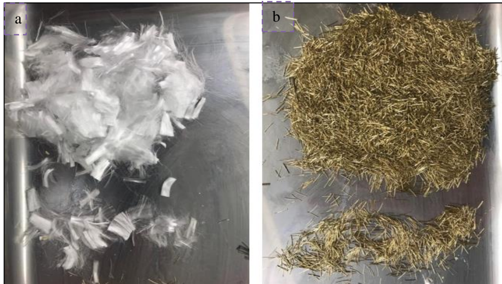
Figure 3.7. a) Polypropylene fibers and b) Steel fibers.
