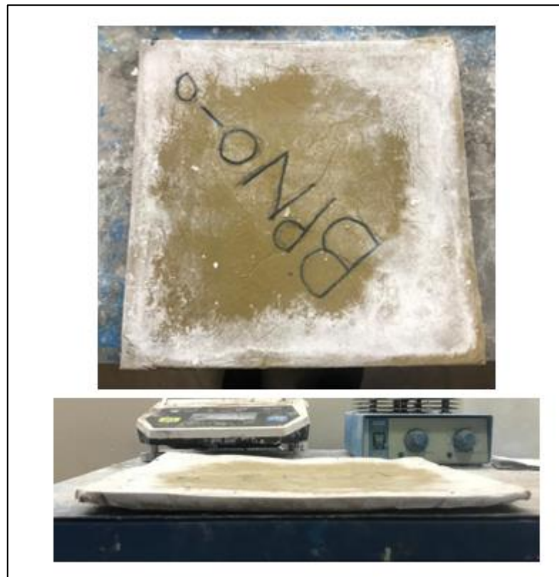
Figure 4.13. a) the surface of WN0-0 batch at the 90 th day of production. b) the deformation of WN0-0 batch at the 90 th day of production.
