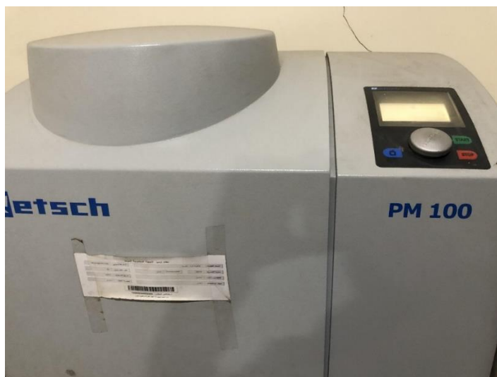
Figure 4.1. A ball mill device used to grind the Ash from burning fuel oil.
