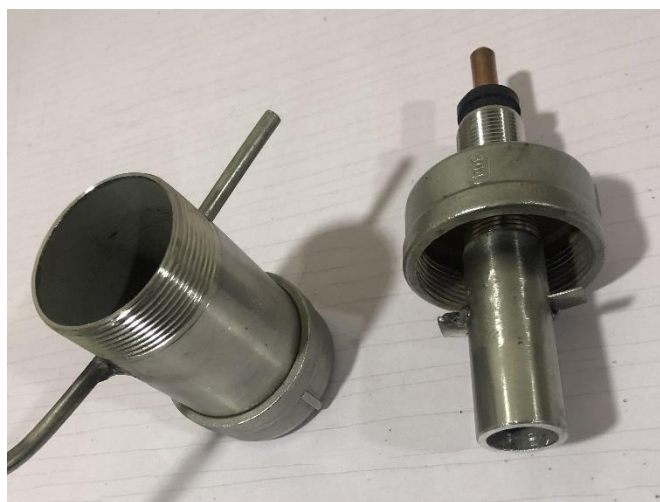
Figure 4.13. A Dow cell that was designed for electrolysis
