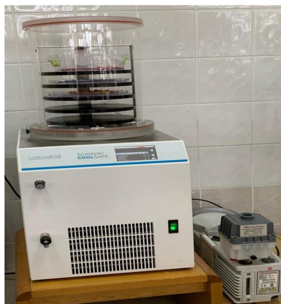
Figure 5.9. Freeze drying of the hawthorn by scanvac coolsafe device.
