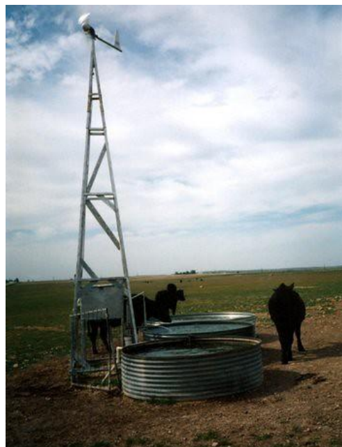
Figure 3.11. Use of small wind turbines to pump water [50].
