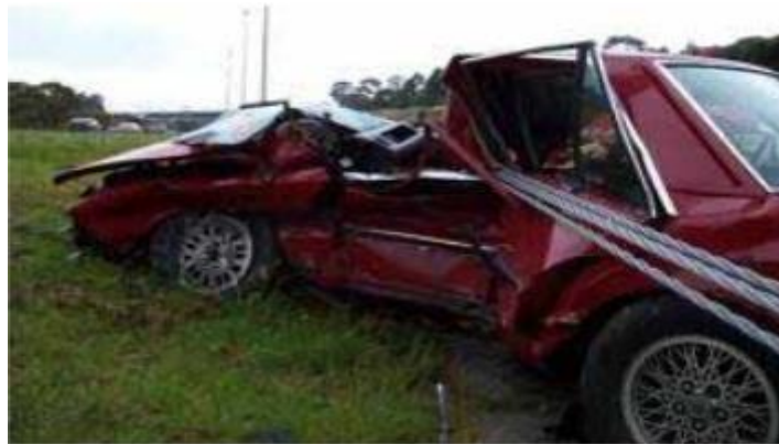
Figure 3.12. Under riding of vehicle due to wire rope [13].
