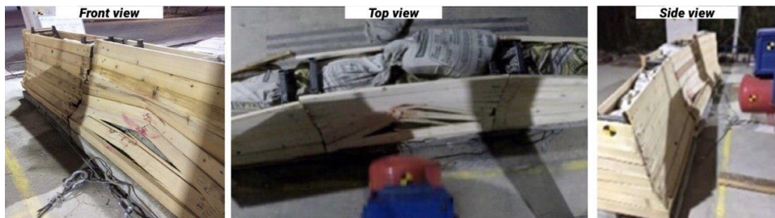
Figure 6.1. Deformation shape of hybrid barrier after crashing with pendulum.
