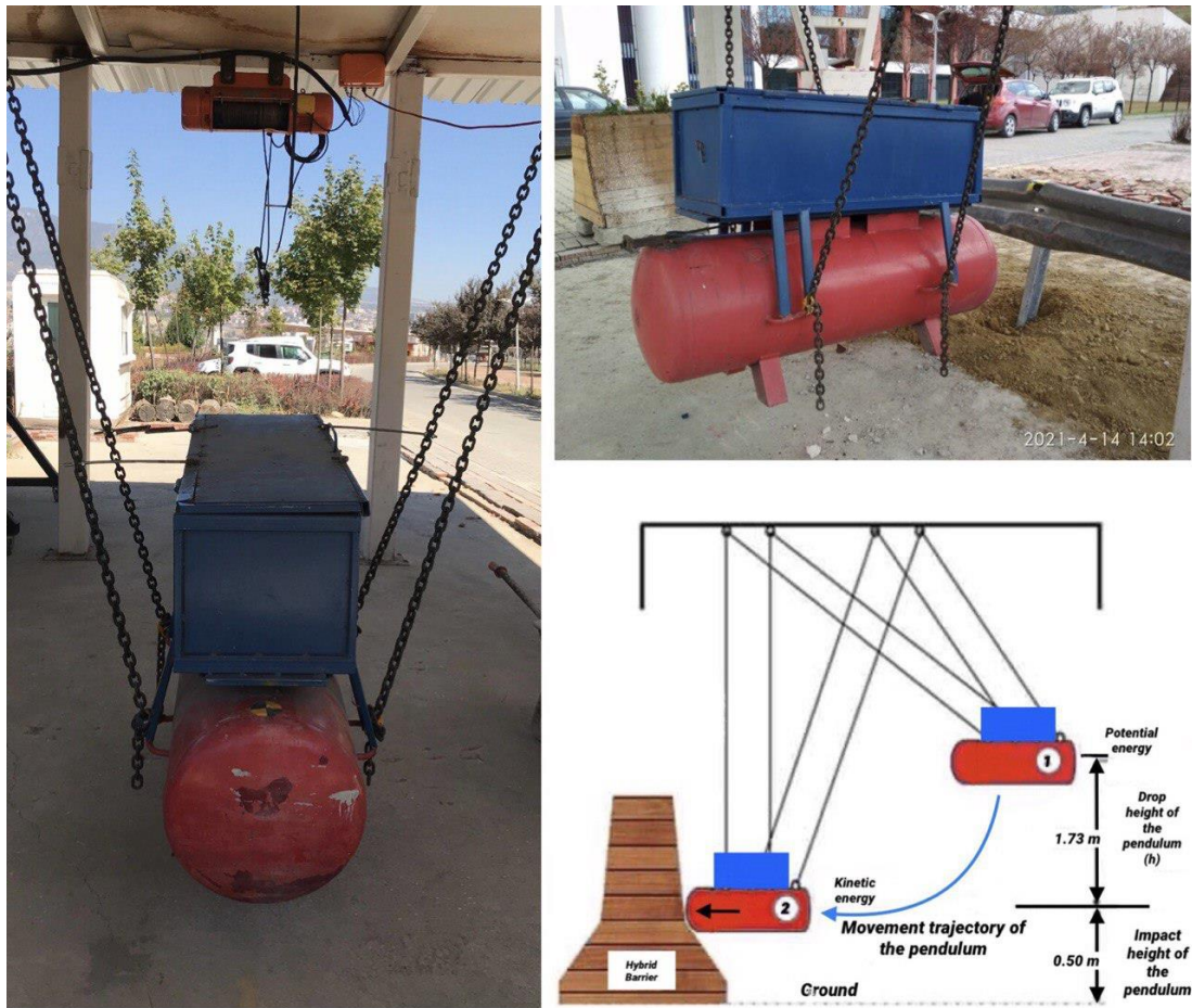
Figure 5.9. Experimental pendulum crash system.
