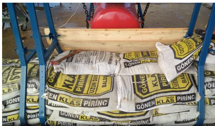
Figure 4.5. Placement of sand inside Hybrid Barrier.
