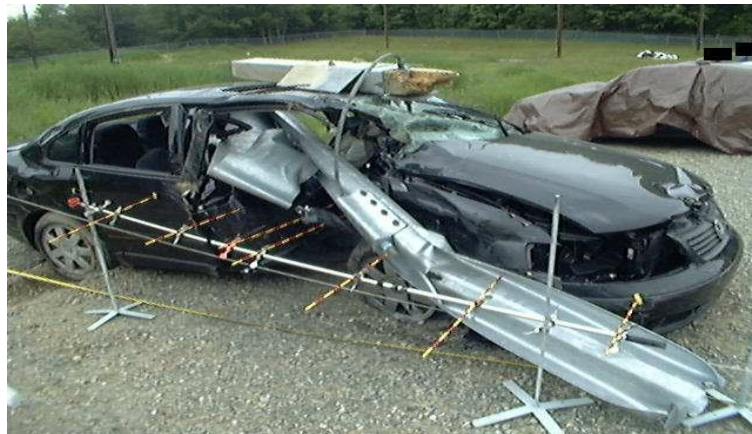
Figure 3.9. Steel guardrails terminal hazards [87].
