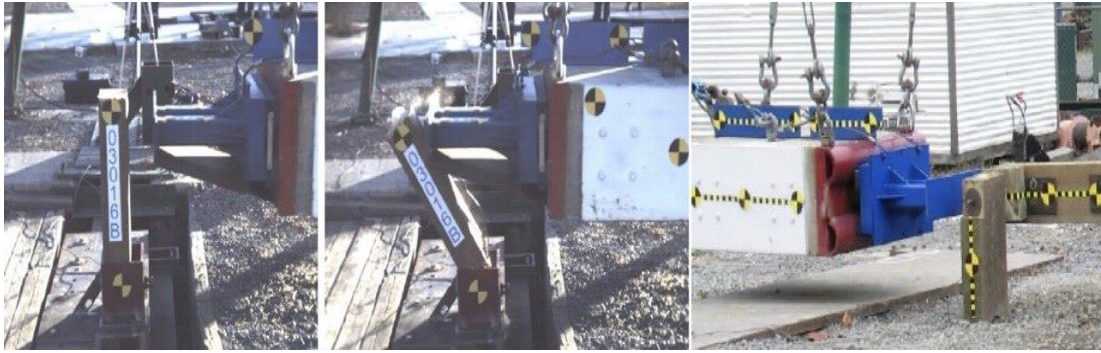
Figure 5.8. Configuration of 2000-kg pendulum used at FHWA and FOIL [128].
