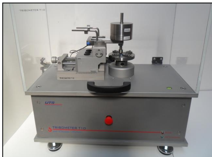
Figure 4.7. UTS Tribometer T10/20.
