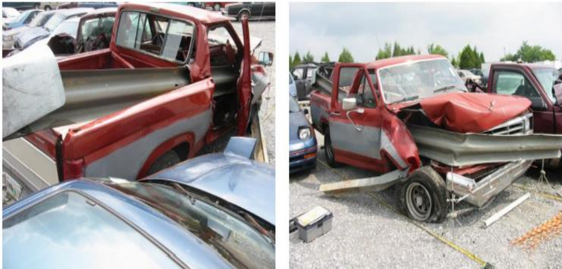
Figure 2.5. Guardrail penetrated the vehicle [59].
