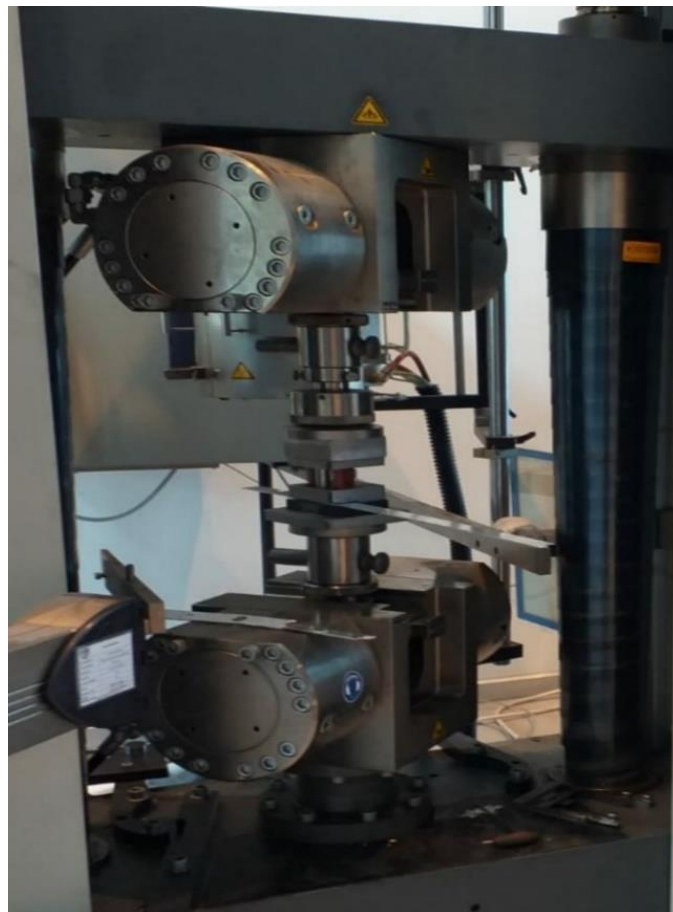
Figure 4.20. Press machine used in piercing process.
