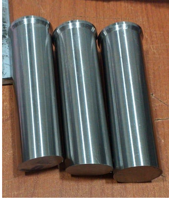
Figure 4.21. Special production punches used in piercing process.
