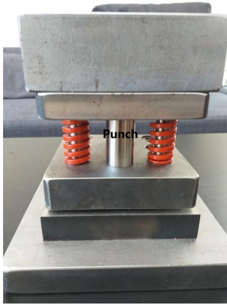
Figure 4.24. Experiment equipment prepared for piercing process.
