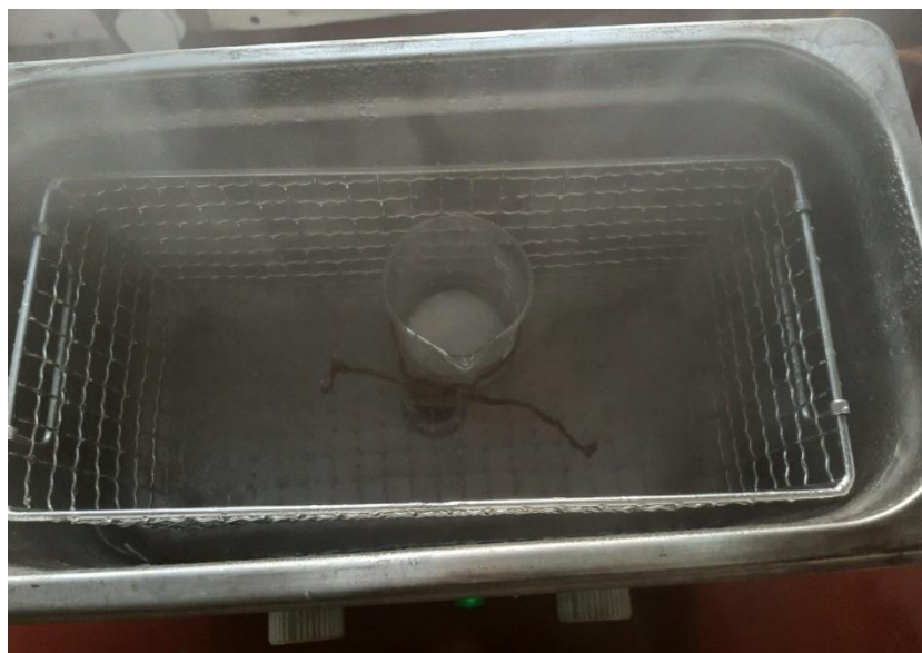
Figure 4.3. The mixing process in ultra-sonic.
