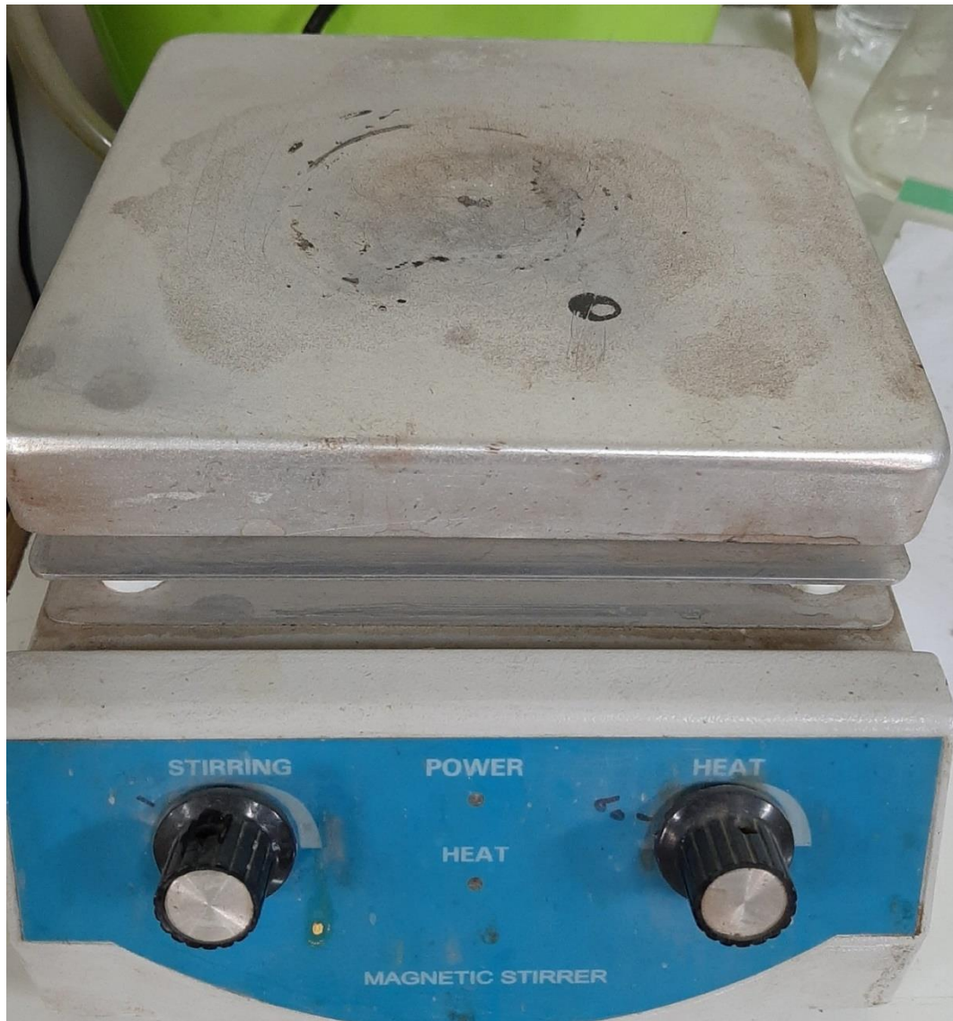
Figure 3.11. Thermal convectector equipped with magnetic drive.
