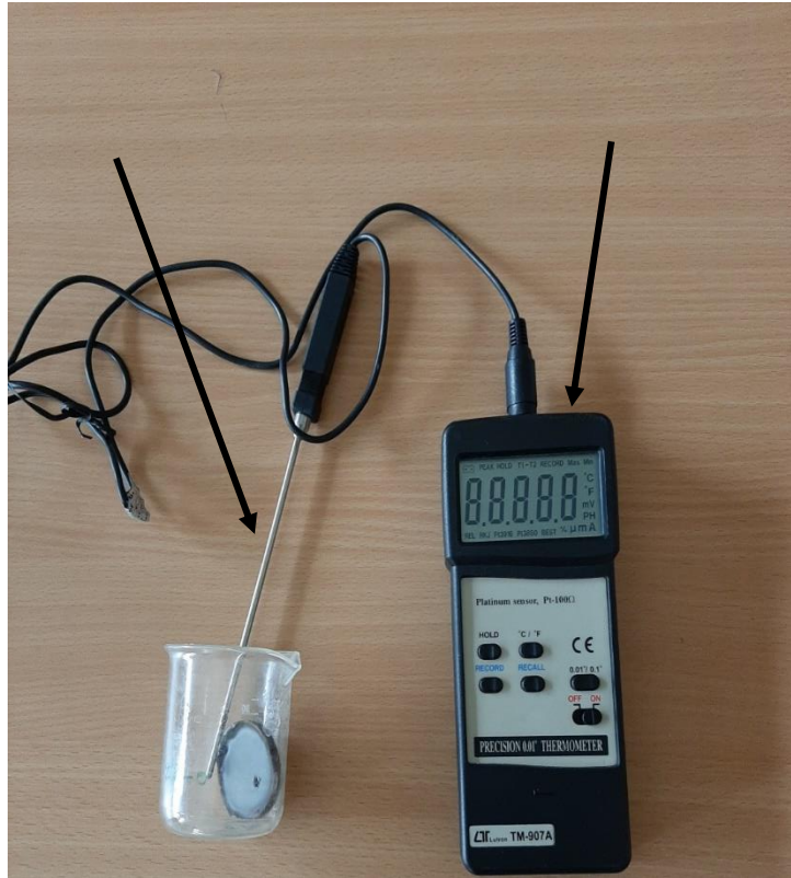
Figure 3.12. Thermocouple sensor and Thermometer.
