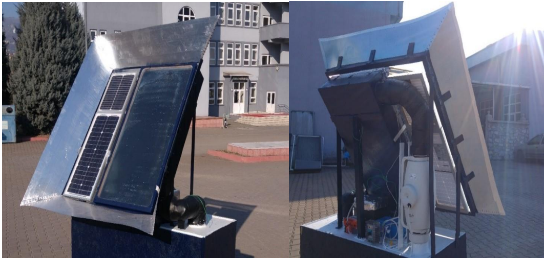
Figure 4.1. Manufactured of concentrated solar air collector with heat store.
