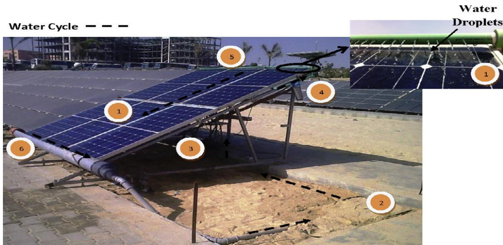
Figure 2.2. Experimental setup 1. PV module, 2. tank, 3. pump, 4. filter, 5. nozzle and 6. drainpipe.
