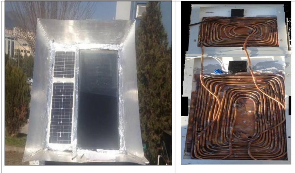
Figure 4.4. the front and rear view of the CPV/T system.
