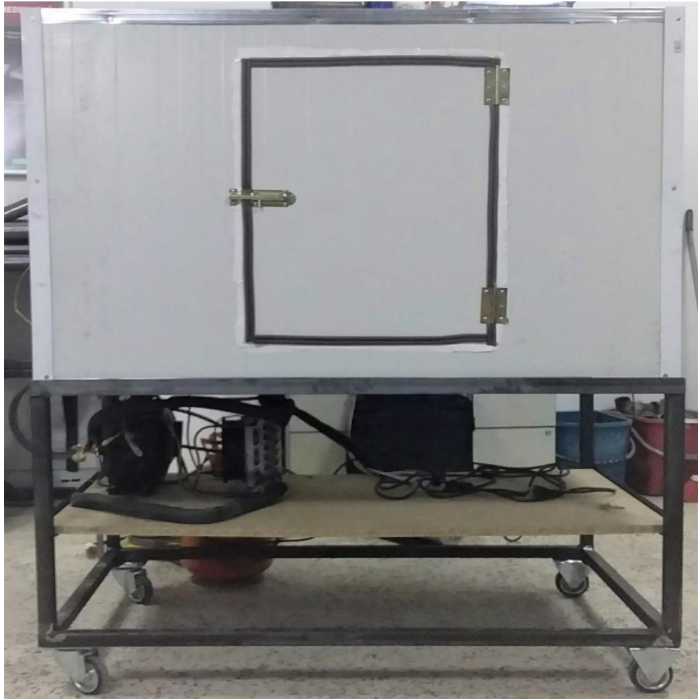
Figure 3.1. The cold storage room compartment.
