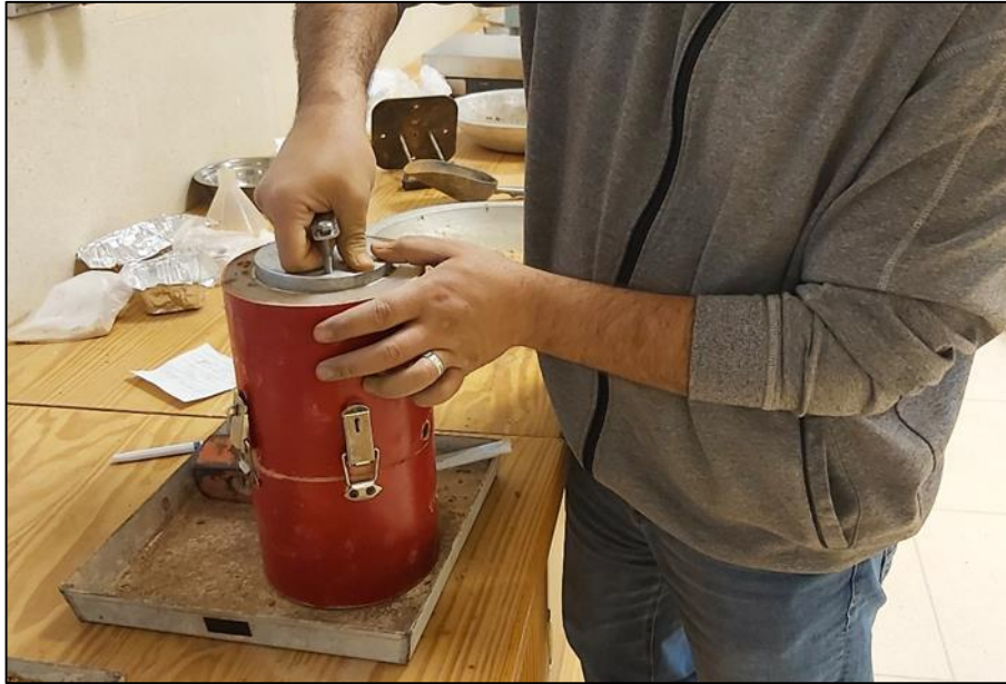
Figure 3.18. The insulation and the removal of the removable plate.
