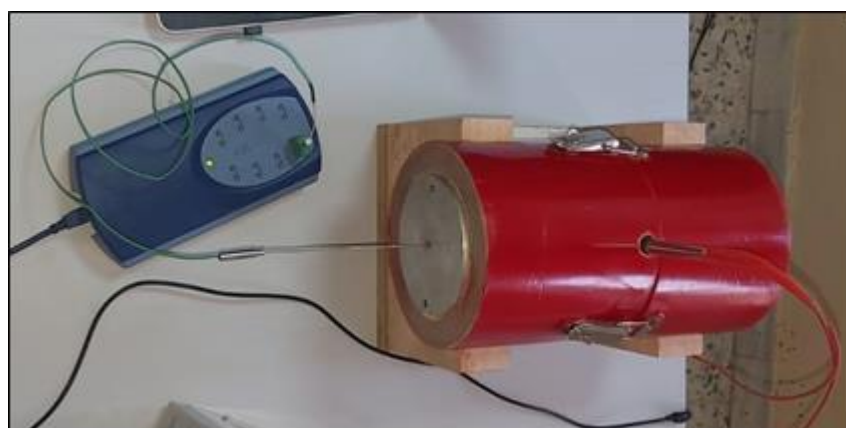
Figure 3.24. The sensor injection inside the cell and the heater injection inside the plate to transfer the heat.
