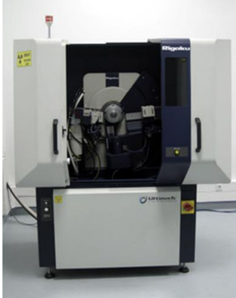
Figure 3.1. Rigaku Ultima IV X-Ray Diffractometer (Karabuk University).
