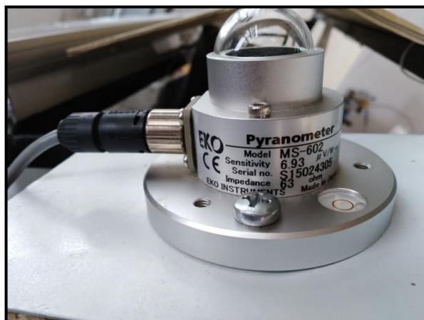
Figure 4.15. Pyranometer used to measure the incident solar radiation.
