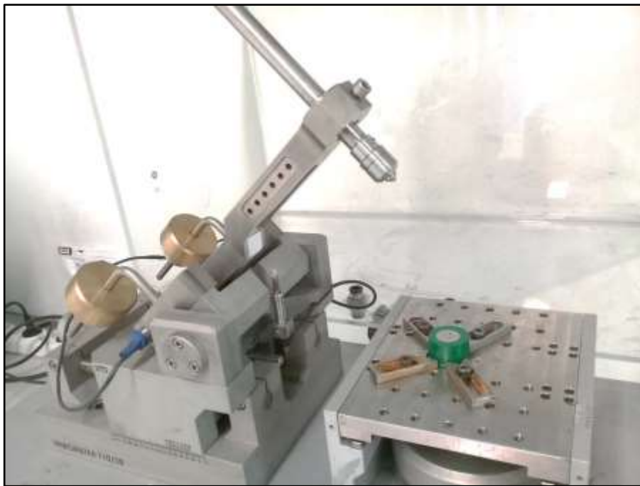
Figure 4.7. Wear test machine (Tribometer).
