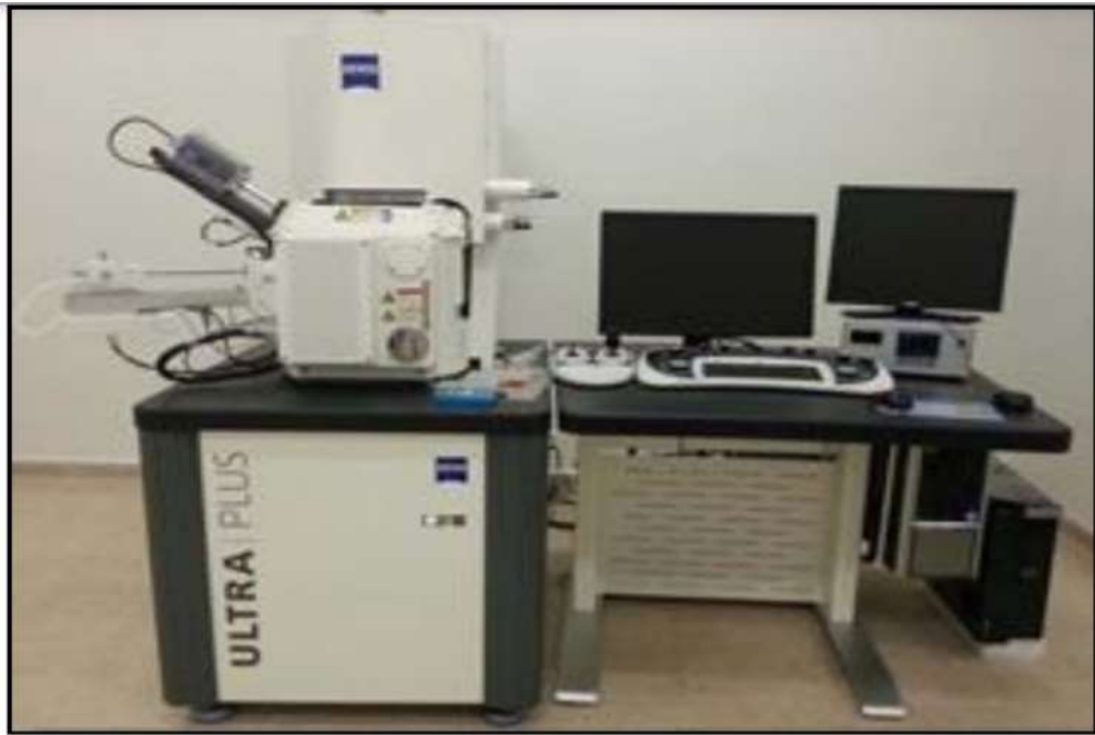
Figure 4.9. SEM device used in the experimental study.
