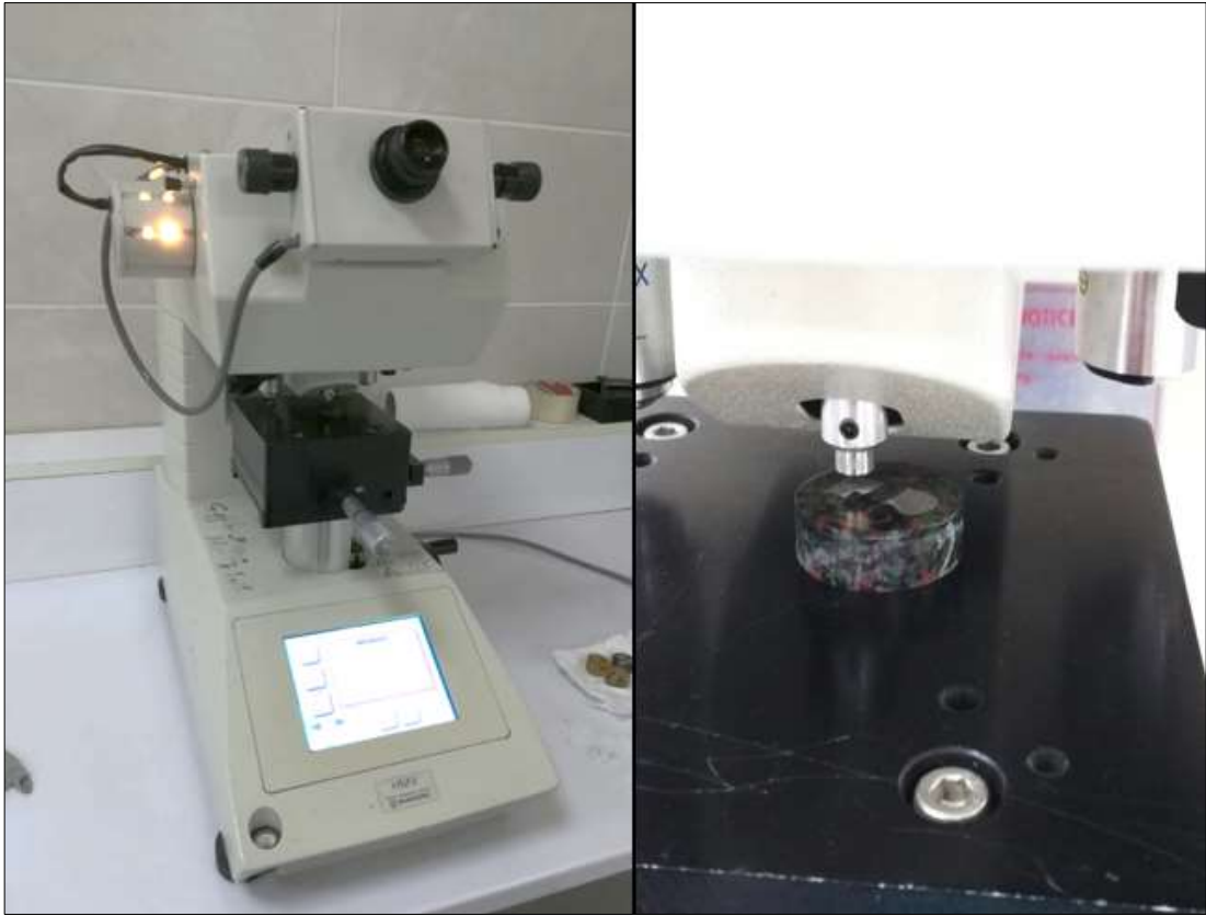
Figure 4.6. Image of microhardness tester for hardness measurements.
