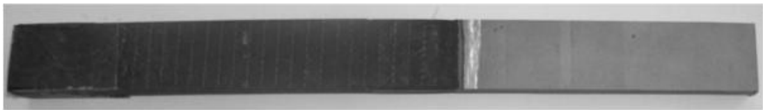
Figure 1.3. Metal–composite specimen produced by hybrid joining [7].
