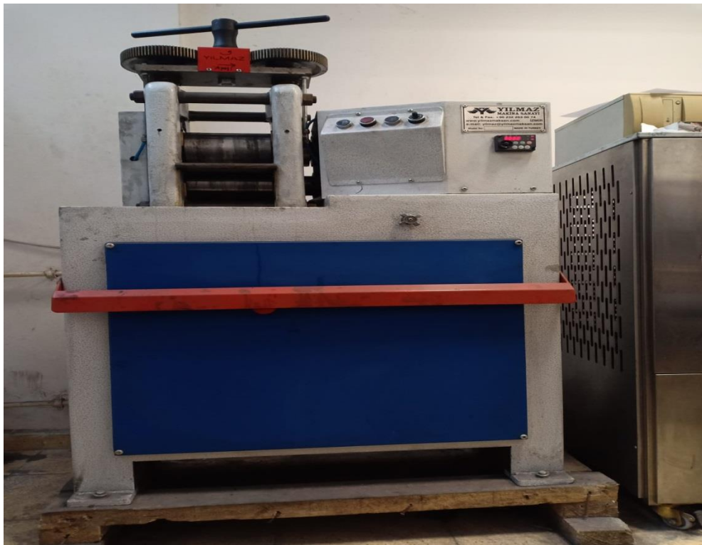
Figure 3.2. Hot rolling machine used for rolling process.
