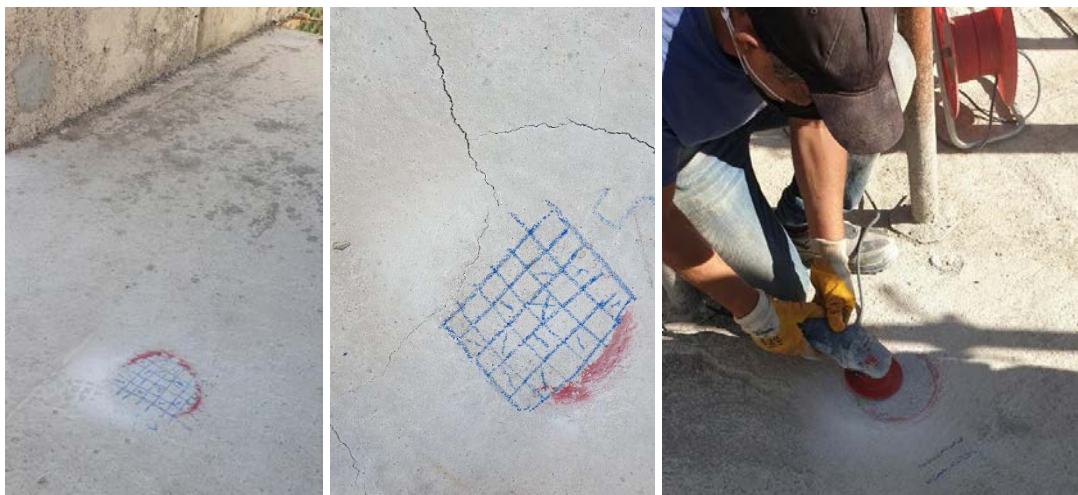
Figure 4. Preparation of grid lines and surface trimming at concrete test hammer points
