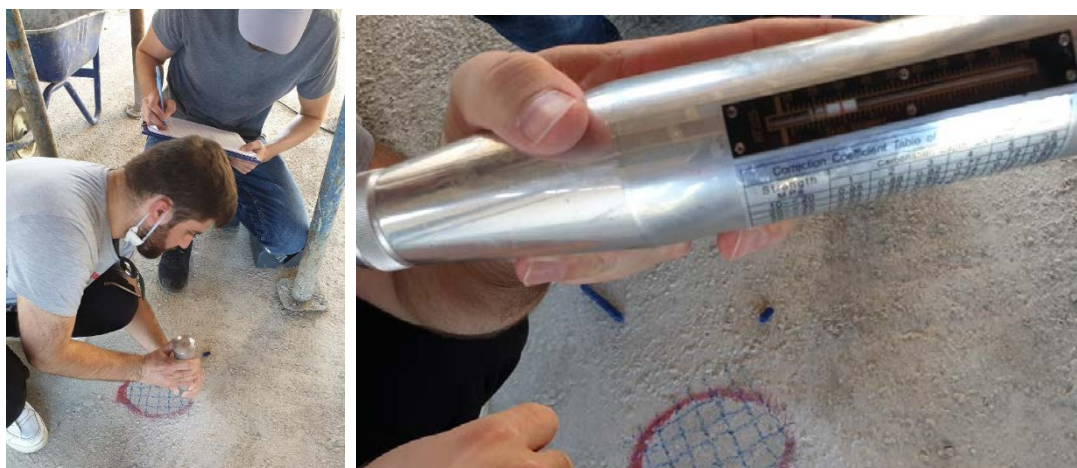
Figure 4. Preparation of grid lines and surface trimming at concrete test hammer points
