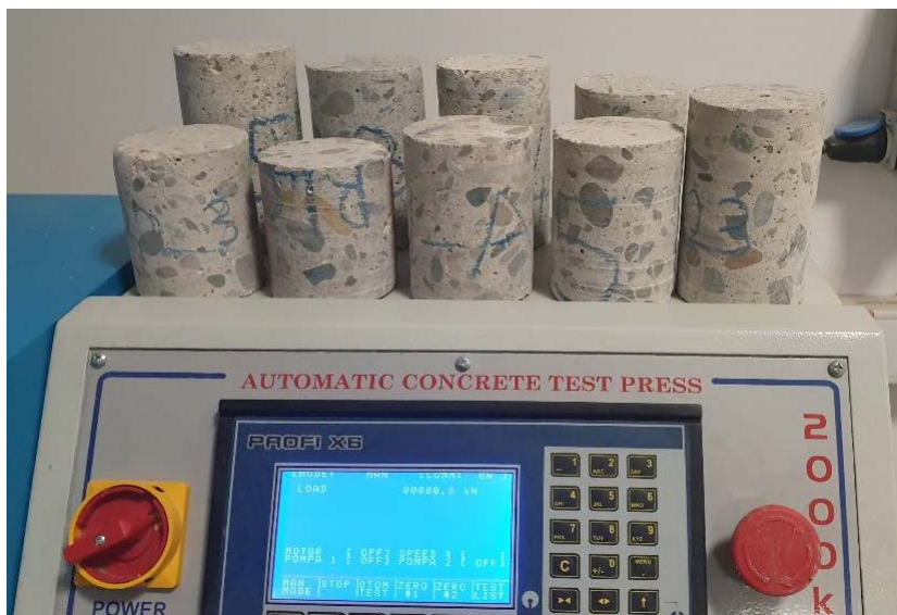
Figure 7. Collective view of core samples on the hydraulic press in the laboratory
