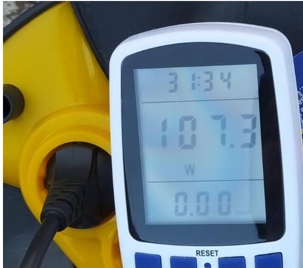
Figure 4.16. Power measurement while plasma is active.
