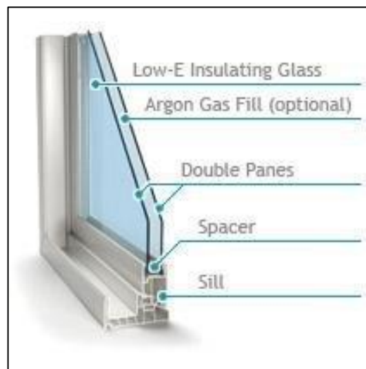
Figure 2.9. Structure of double glazed window (Lohia and Dixit, 2015).
