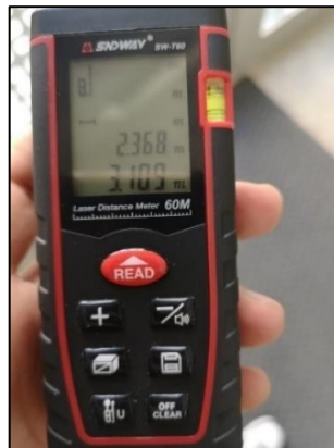
Figure 3.5. SNDWAY SW-T60 Laser distance meter.
