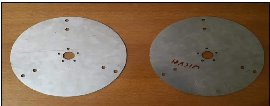
Figure Appendix C.9. Iron Discs Connecting Struts to the Shaft.
