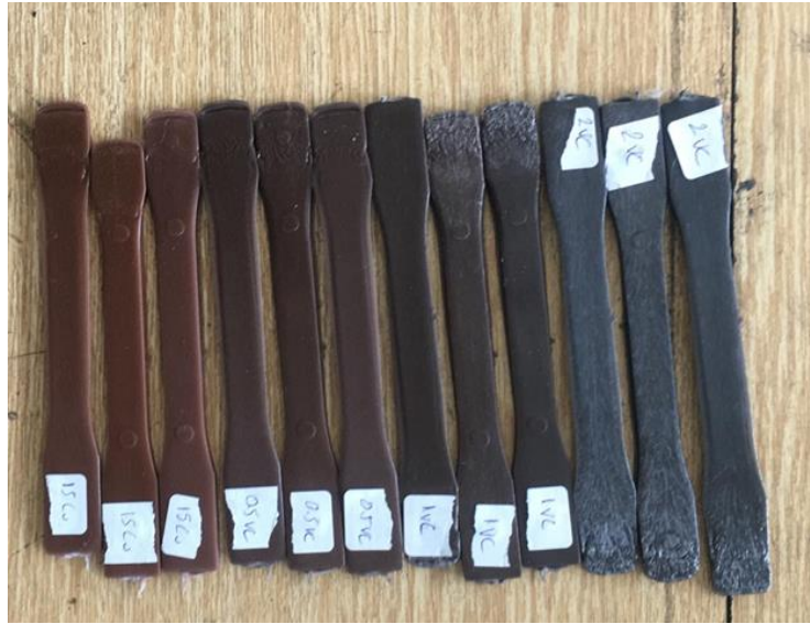
6.1. Produced dog-bone shaped samples.
