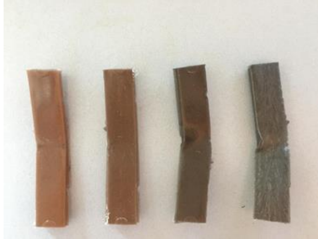
6.3. Samples after impact test.
