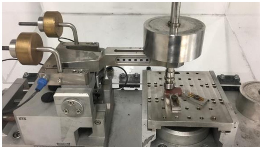
6.4. Image taken during the wear test.
