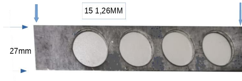
Figure 5.14. Dimensions of punch geometry (length 151.26mm, width 27mm).
