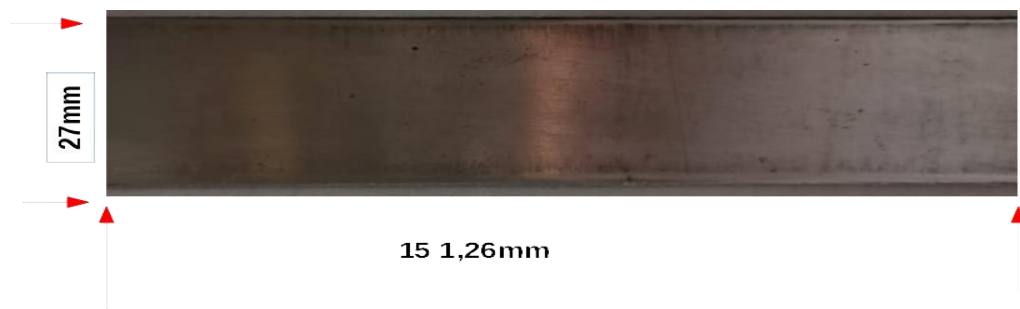
Figure 4.11. Dimensions: Thickness 3mm, length 151.26mm, and width 27 mm.
