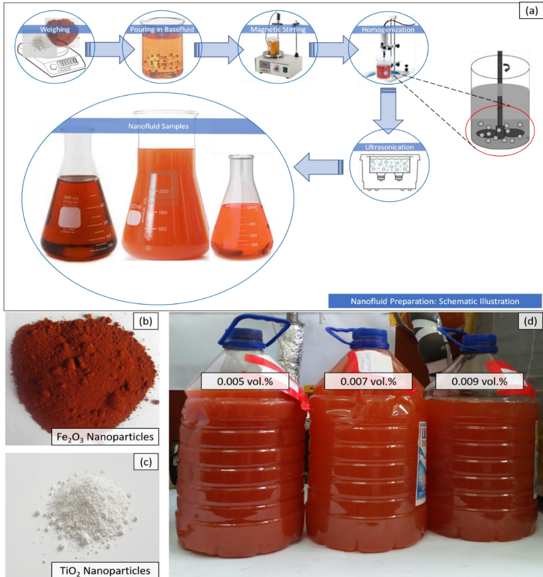
Figure 1.3. Preparation of nanofluid in bulk quantity through two-step nanofluid preparation method (a) nanofluid preparation steps, (b) ferric oxide nanoparticles, (c) titanium dioxide nanoparticles, and (d) produced nanofluid in container [7].
