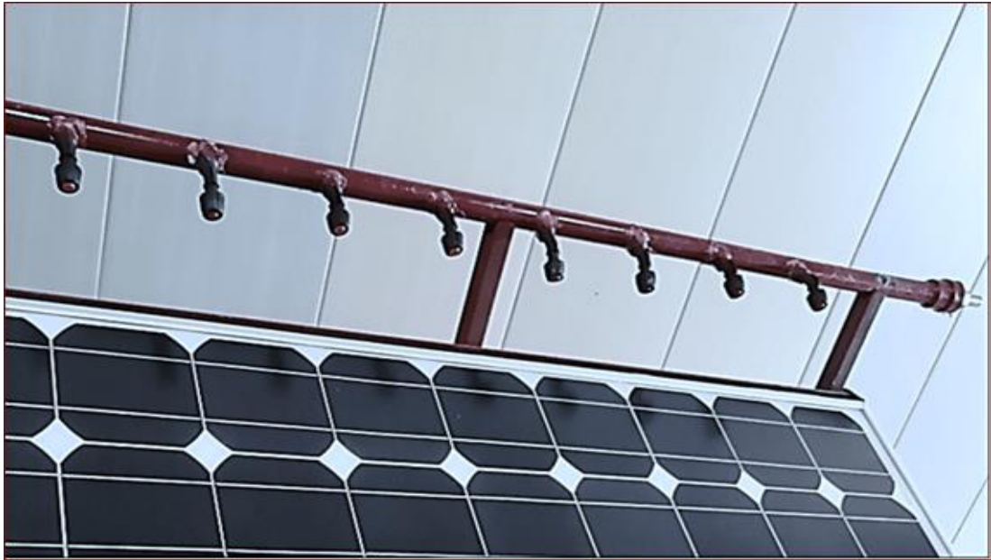
Figure 3.15. Experimental setup module upper cooling technique nozzles.
