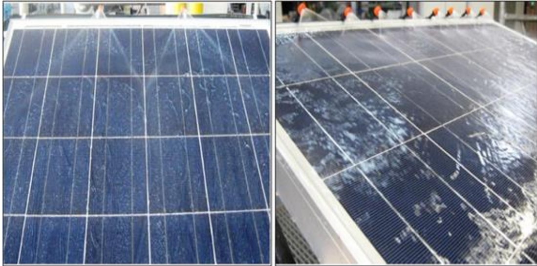
Figure 2.19. Diversity of number and design of the angles PV panel nozzles [41].
