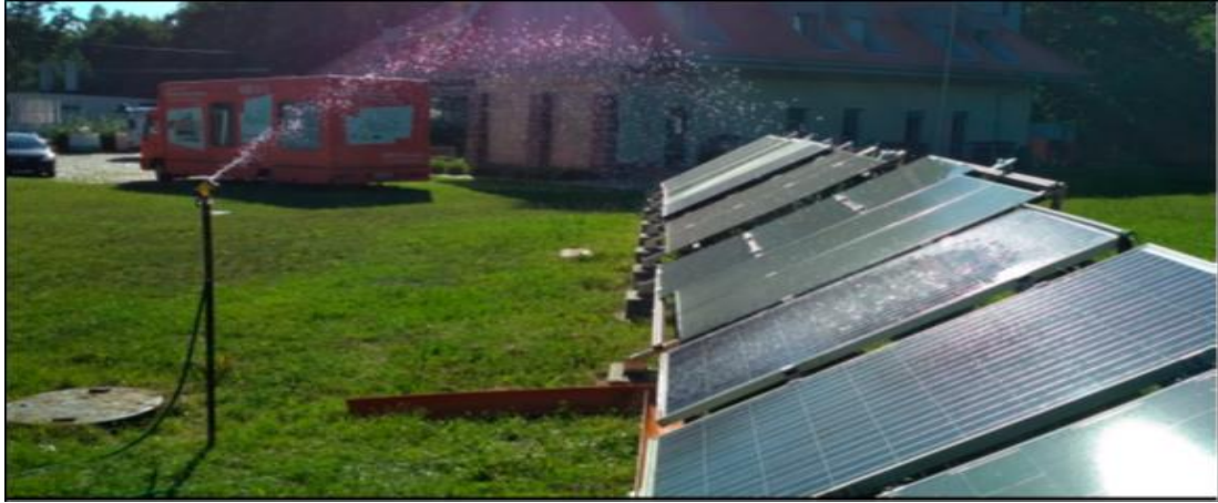
Figure 2.25. Cooling of PV array by atomization of rain [56].
