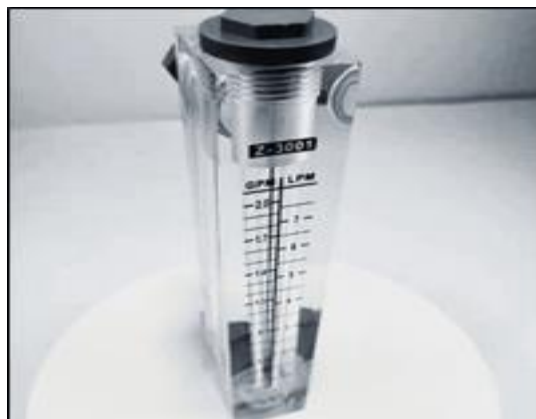
Figure Appendix 3. Flow Meter.
