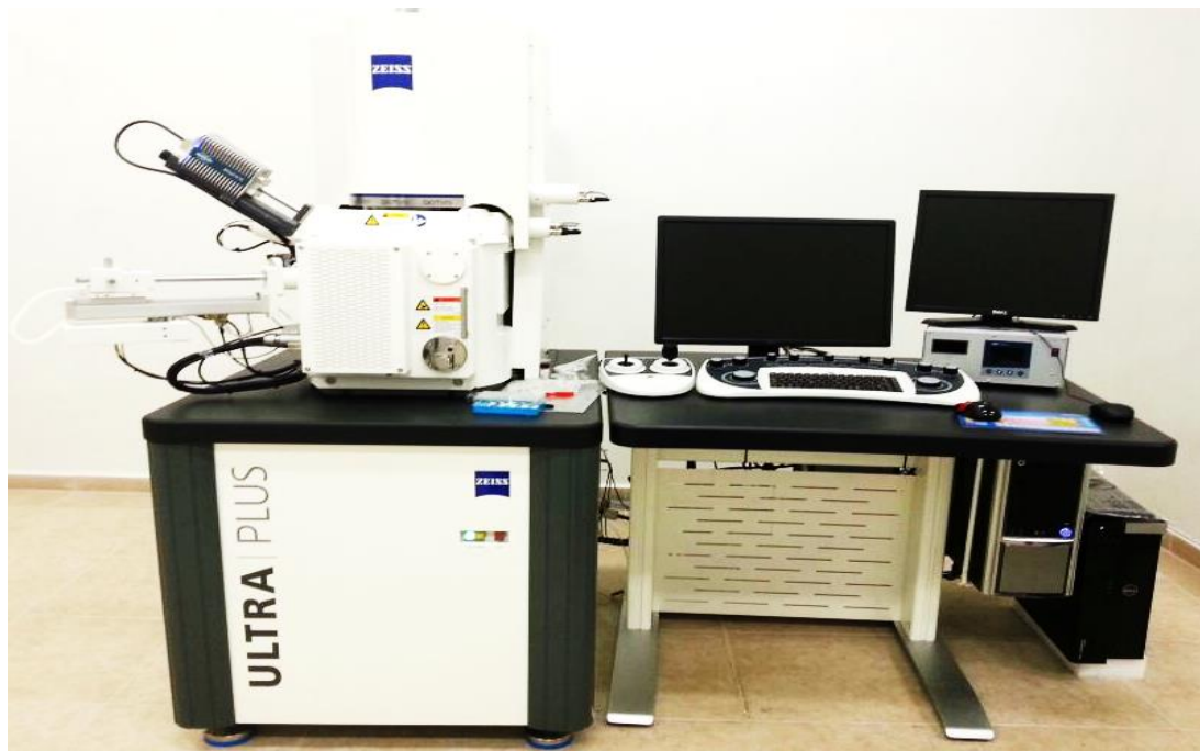
Figure 3.6. Scanning electron microscope used for microstructure investigation.
