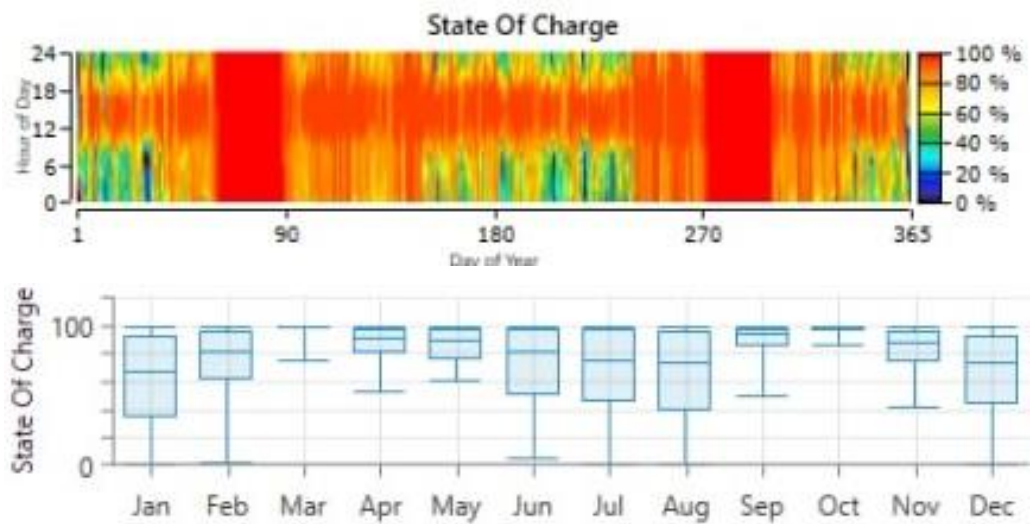
Figure 5.24. Charge of the battery for Fallujah.
