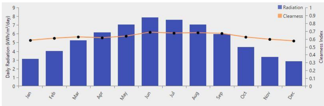
Figure 3.18. Monthly average solar irradiance and clearness index for Fallujah.
