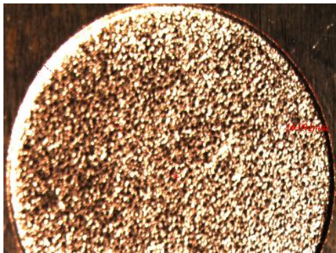
Figure 5. 12 Microscopic image of machined hole, minimum OC at process parameters E1A2B1C2.
