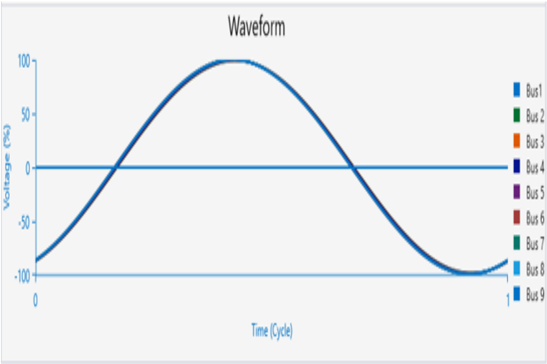
Figure 4.14. Voltage waveform of all buses without PV connection.
