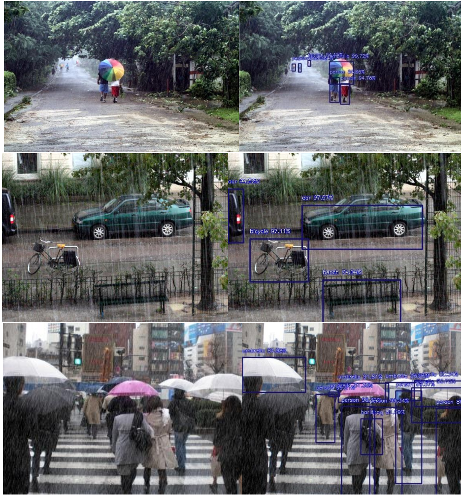
Figure 5.10. Experimental results of YOLOv3 model on real rainy images.
