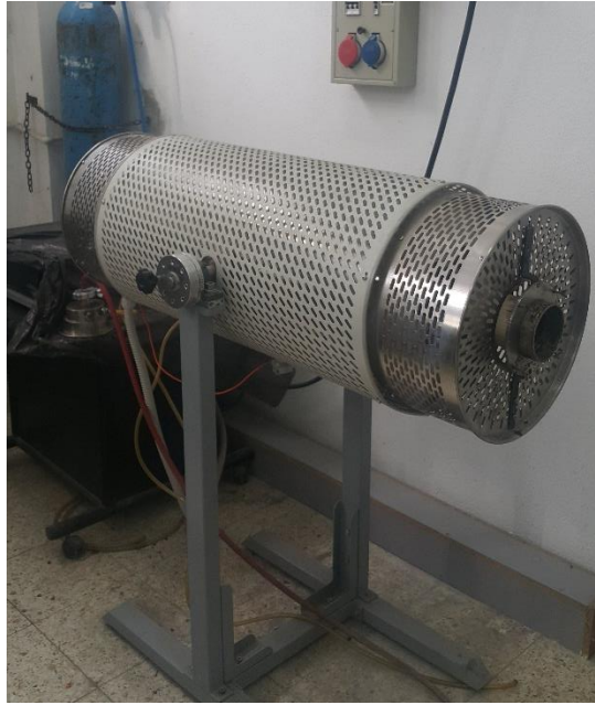
Figure 4.3. Atmosphere-controlled tube furnace.
