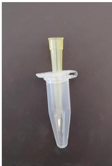
Figure 3.2. A small hole was made in the lid of an eppendorf microcentrifuge tube.
