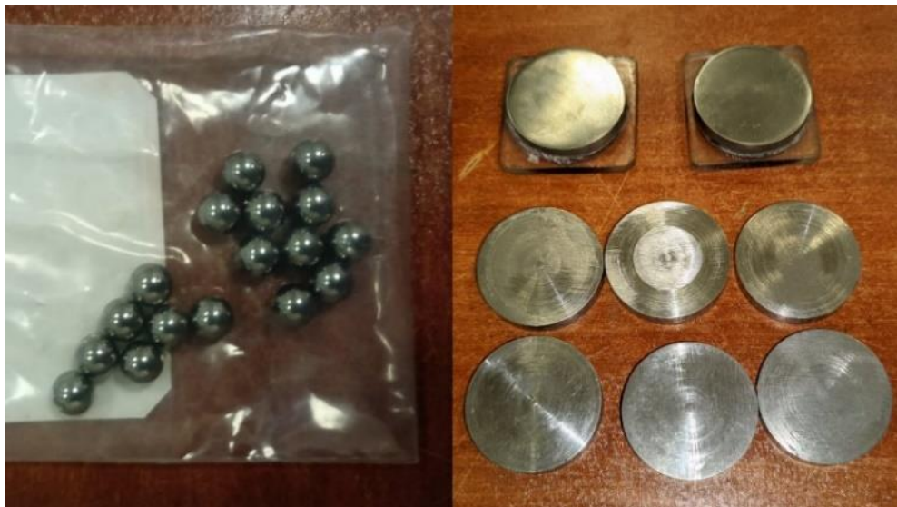
Figure 4.1. WC cemented carbide balls and Ti-6Al-4V specimens.
