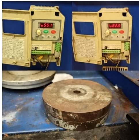
Figure 4.6. Load varieties of 10-20 N and sliding speeds of 50 and 75 mm/s.
