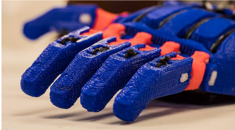
Figure 2.10. Prosthetic limb made using FDM technology.
