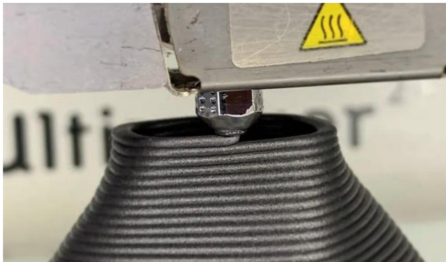
Figure 2.1. Build layers one on top of the other [29].
