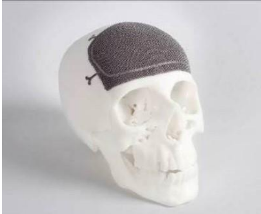
Figure 2.6. Skull Brace made by EBM metode [34].
