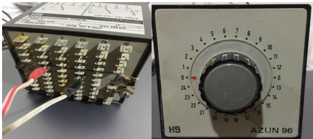
Figure 3.11. Utilized selector switch.
