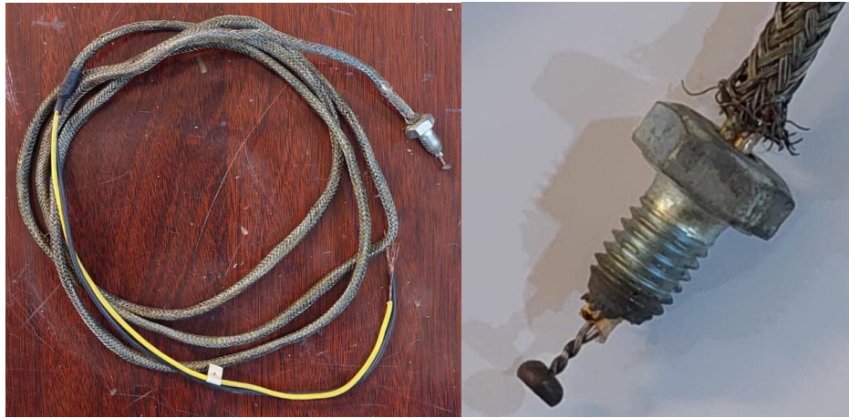
Figure 3.9. Thermocouple utilized in the present work.
