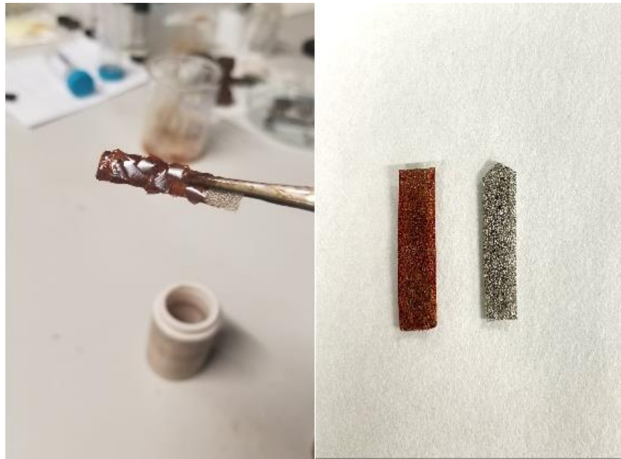
Figure 5.6. Macro view before and after CFO coating with hydrothermal method.
