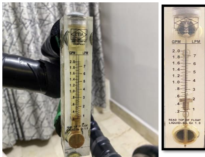
Figure 4.15. Flow meter of water.
