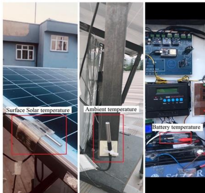
Figure 3.8. DS18B20 temperature sensor.
