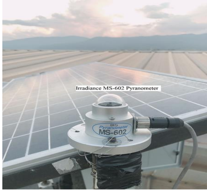
Figure 3.6. MS-602 pyranometer sensor.
