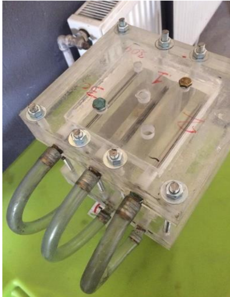
Figure 0.6. Testing of alkaline electrolysis cells stack
