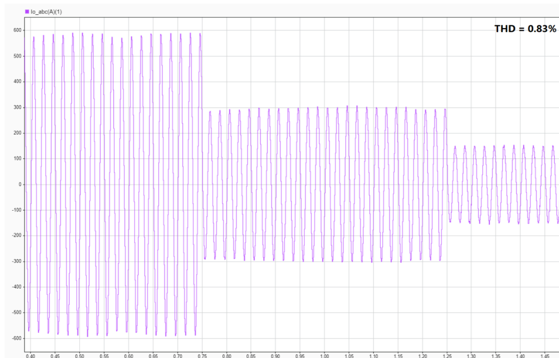
Figure 4.10. THD for MPC controller.
