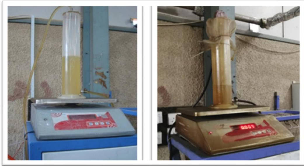
Figure 3.5. The unit of fuel flow rate measurement.
