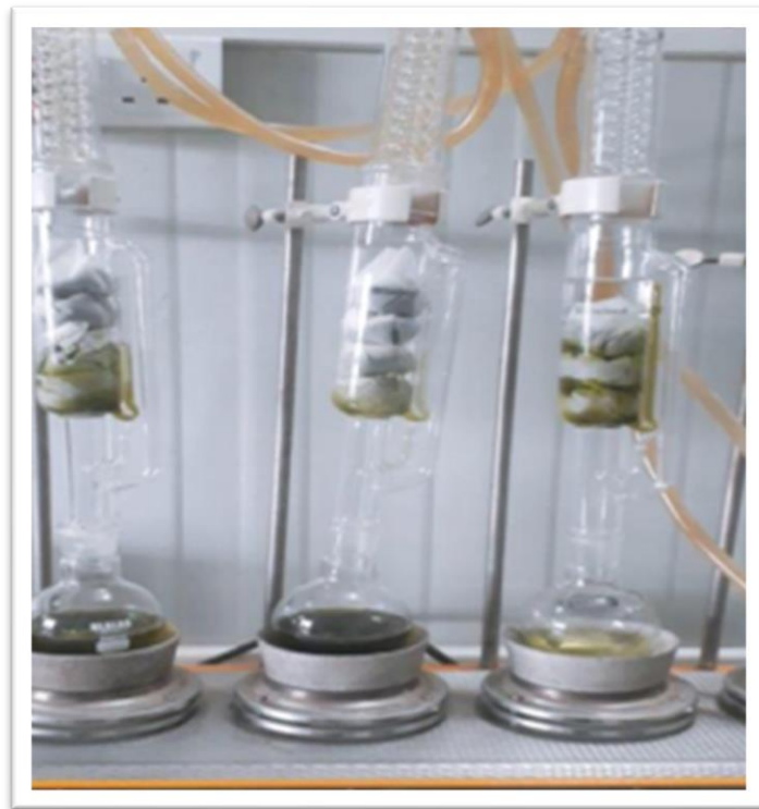
Figure 3.18. The soxhlet apparatus [57].
