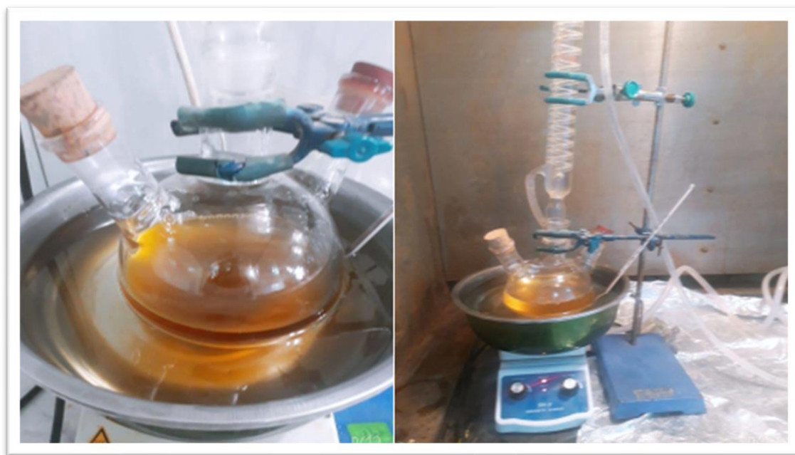
Figure 3.19. A water bath with 3-neck flask has a capacity of 1 Liter
