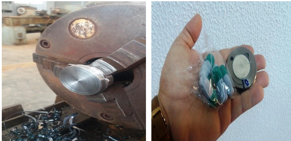
Figure 3.3. Plate Metal to Prepare it For Steps of Measurements of X-Ray Diffraction [Author image].
