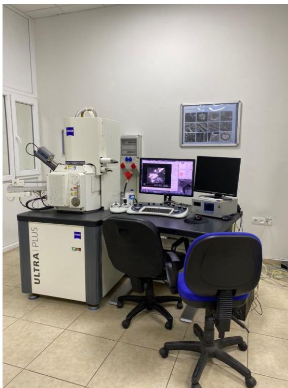
Figure 5.4. Scanning electron microscope (SEM).
