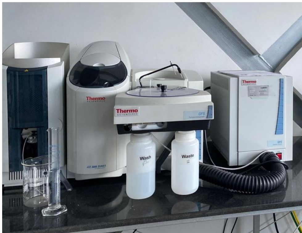
Figure 5.7. Atomic absorption spectroscopy (AAS).
