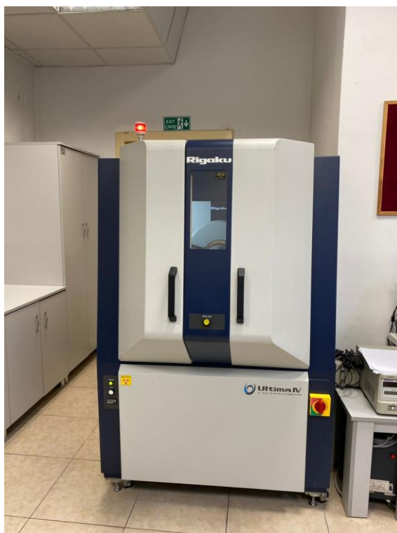
Figure 5.2. X-ray diffraction instrument (XRD)
