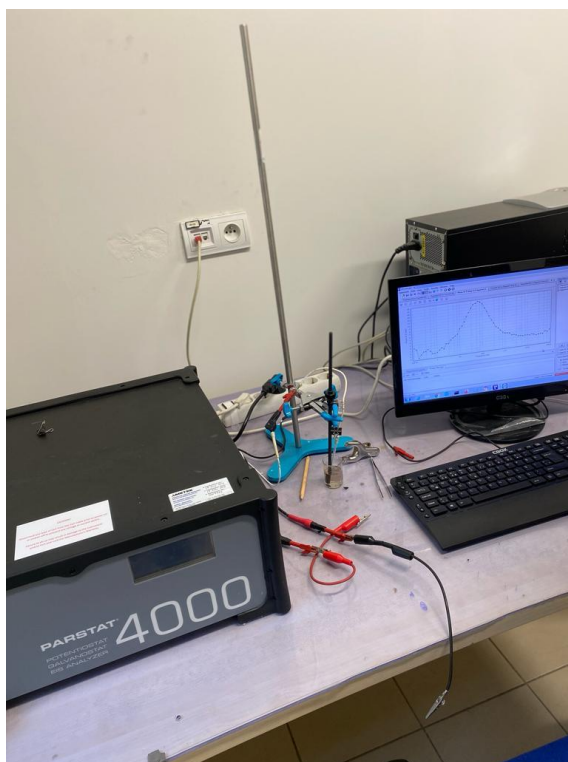
Figure 5.8. Electrochemical measurement device.
