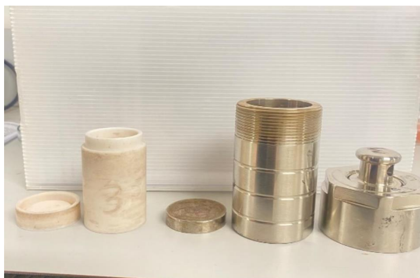
Figure 5.7. Teflons and autoclaves used in the hydrothermal process
