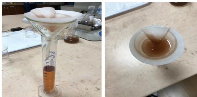
Figure 3.6. Filtering the solution through filter paper.
